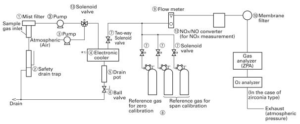
\*1) Be sure to use a dehumidifier such as electronic cooler for NO, SO₂, and CO analyzers of 0 to 200 ppm range (≒2°C saturation or lower).
